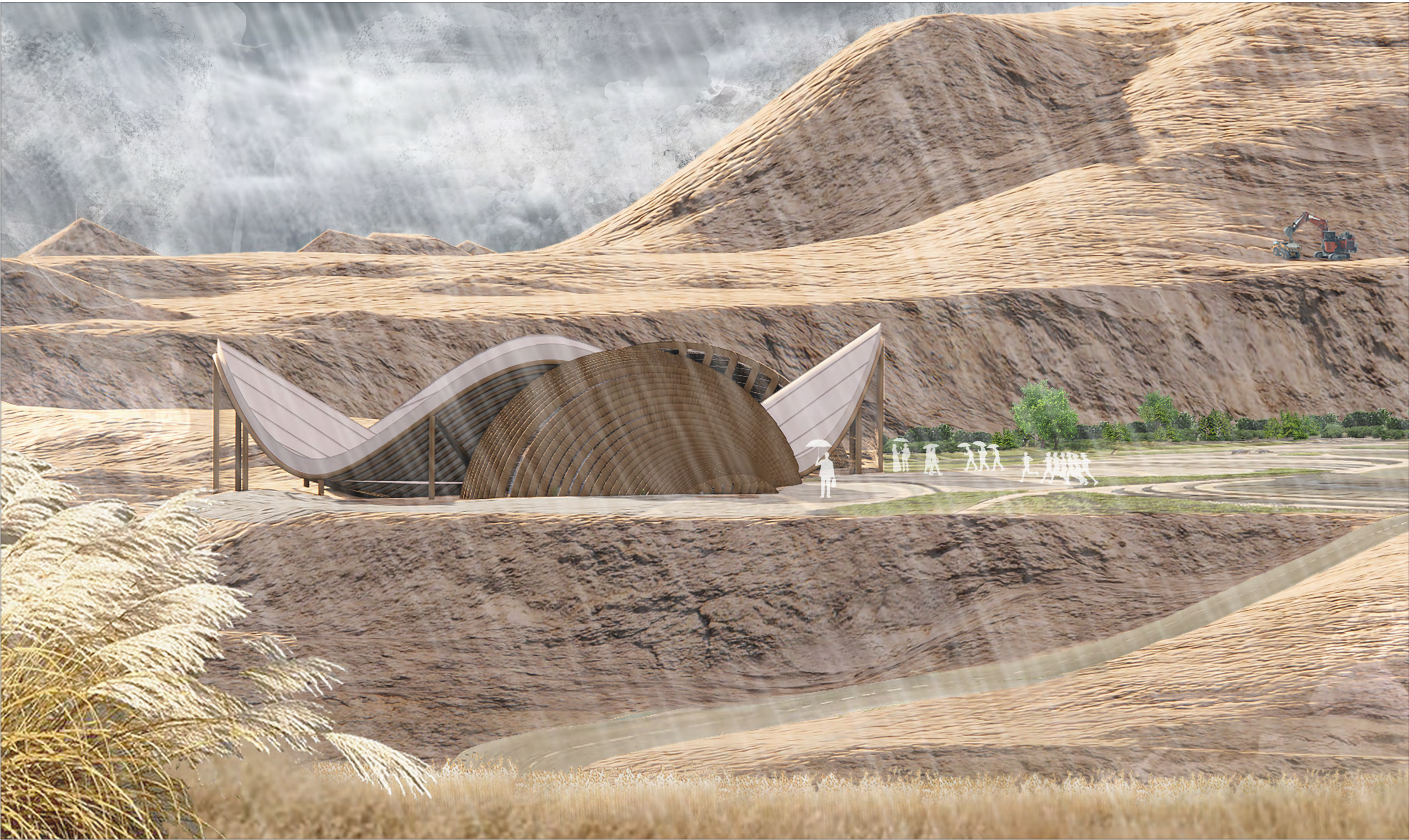
During rainy season the building’s roof harvests the rainwater to maintain the plants within the greenhouses.
